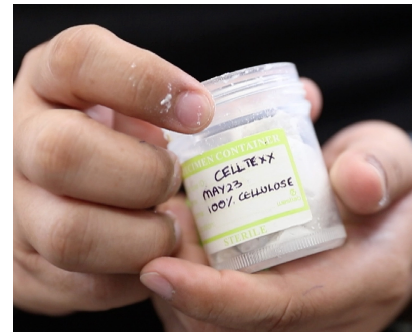
POWDER - CELLULOSE IS DRIED INTO A POWDER.
